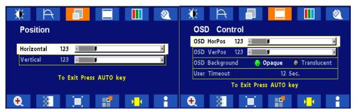
Push "Up" or "Down" button to select between "Horizontal" or "Vertical" then push "Select" Use "Left" or "Right" button to adjust Push "Up" or "Down" button to select between "OSD Hor. Pos.", "OSD Ver. Pos.", "OSD Background", or "User Timeout" then push "Select"
